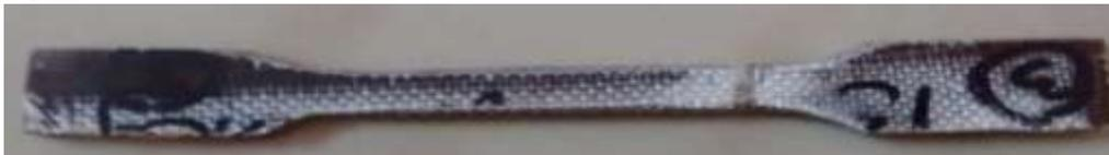
*Fig: 8 Fracture occurred with Brittle behaviour*
