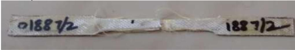
*Fig: 10 Fracture occurred with no Delamination*
