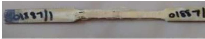
*Fig: 6 Fracture occurred with Delamination behaviour*
